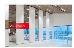
Quickly opened, quickly closed: with ComfortDrive, the elements move quickly to the desired position, monitored by Smart Control.
